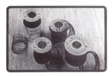
These Round Abrasive Cords and Flat Tapes will finish surfaces that are inaccessible to most conventional tools. These flexible abrasive cords and tapes will deburr, grind and polish those hard-to-reach holes, slots, grooves and curved surfaces. Aluminum Oxide is suggested for use on ferrous metals; Silicon Carbide for non-ferrous, plastic and wood; Crocus for final polishing.
